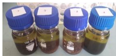
Fig. 2. Four aqueous extracts made from olive cakes: 1- Arbequina, 2-Palomar, 3- Agro Igualada, 4- Polpa d'oliva, by ultrasound for 1 hour, at pH = 2
